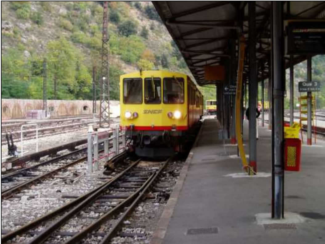
CD-11: French National Railways (SNCF) narrow-gauge, third-rail electric Le Petit Train Jaune at Villefranche/Vernet-les-Bains (2003/10/13) [PETER DAWES].
